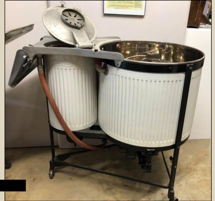
Twin Tub "Easy" Washing Machine with vacuum cup technology. Syracuse Washing Machine Company. Donated by the Walt Benton Estate. Circa 1920-1932.
