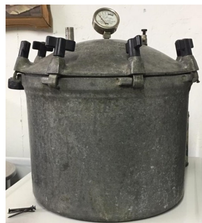
This 1930's pressure canner has seven wing nuts holding the lid in place and a gauge to show the pressure level. Do you remember having your gauge tested at the Extension office?
